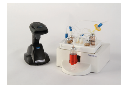
Modular-Lab eazy with cassette and barcode reader
